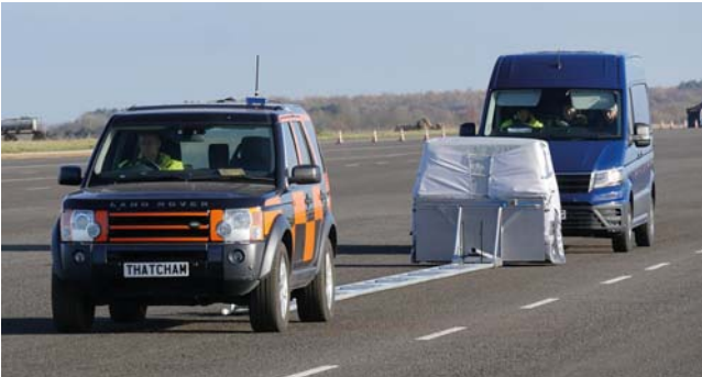
VW Crafter demonstrating high-speed emergency braking while following Thatcham Research towed target car
