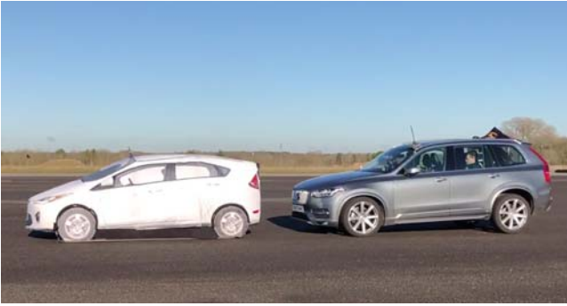
Volvo XC90 demonstrating high-speed emergency braking while following Thatcham Research remote-controlled target car
