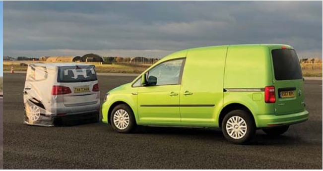
VW Caddy demonstrating low-speed emergency braking while approaching Thatcham Research static target car
