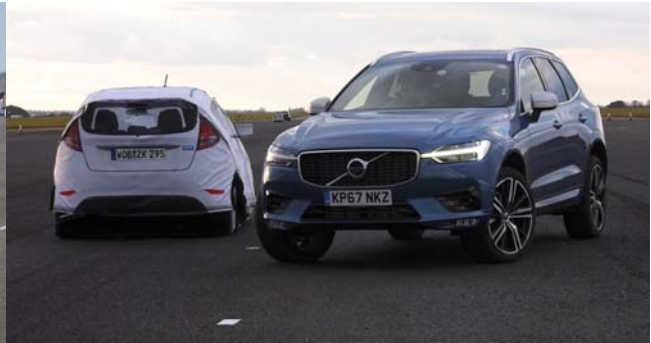
Volvo XC60 demonstrating turn-across-path prevention system while approaching Thatcham Research remote-controlled target car
